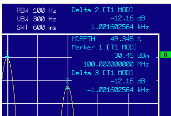
Fig. 5-17 Measurement of the AM modulation depth. The modulation depth shown is MDEPTH = 49.345%. The frequency of the AF signal can be obtained from the frequency display of the delta marker.
